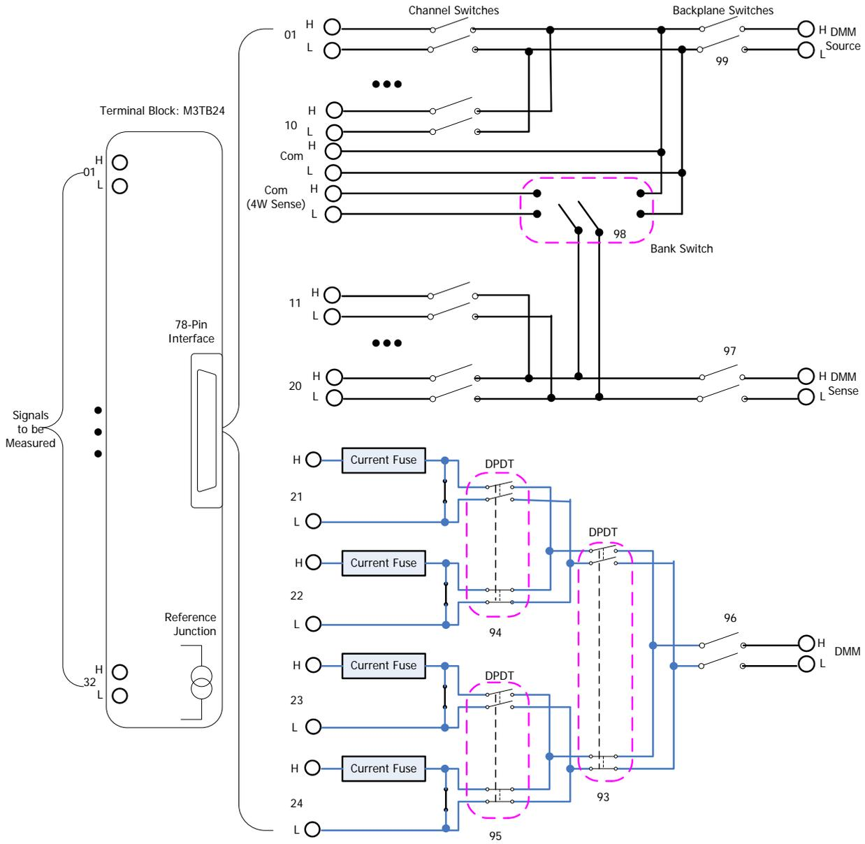
Figure 5-5 MC3324 Schematic Diagram
